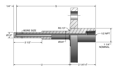
("U" length for non-lagging wells) = "S" - 2" ("U" length for lagging wells) = "S" - 2" - "T" (To solve for "T"), "T" = "S" - "U" - 2" (When "U" and "S" are specified)
